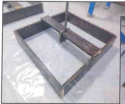
2. Spacer and pulling system positioned in frame work
