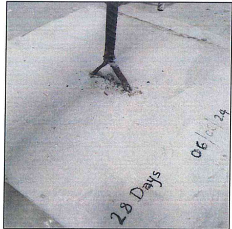
5. Sample after pull out test
